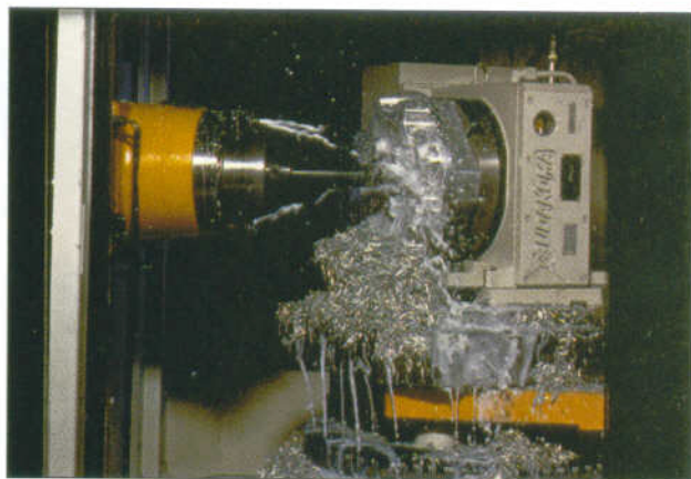
Figure 8.16 CAD Data Used Directly by Machine Tool This computer-numeric-control (CNC) machine tool can interpret and process 3-D CAD data for use in manufacturing, to create dimensionally accurate parts. (Courtesy of Intergraph Corporation.)
